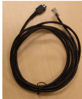
Remote cable ST40 connector to RJ45
